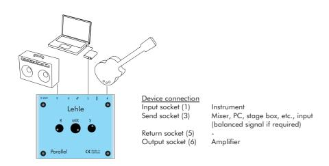
A further, entirely practicable use of the Lehle Parallel M is as an active DI box. The unfalsified signal is then routed via the Send socket (3) to the input of a mixer, stage box or an A/D converter or sound card, while the accustomed sound can be heard simultaneously from the amplifier.
