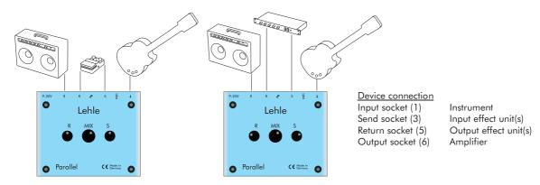
Without a Lehle Parallel M, injecting effects into the signal path can cause all kinds of problems, especially if you're using older, so-called "vintage" effects which, as every player knows, produce a unique sound, but generally falsify the original signal very noticeably. The Lehle Parallel M will help you here in several ways:
