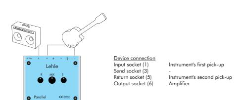
Many instruments have two different types of pick-up, such as one magnetic and one piezo pick-up, for example. The Lehle Parallel M is excellent at mixing these signals.
